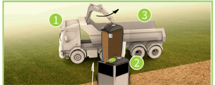
1. Truck with crane 2. Lift the bag 3. Empty the bag
